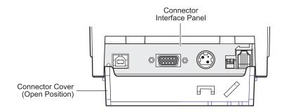
*Caution:* Connect the cables to the printer before applying power. The host computer should always be turned off before connecting communication cables.
